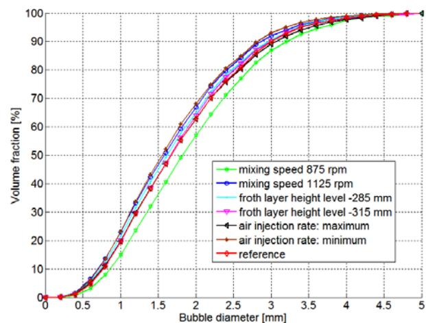
Figure 4. Effects of froth layer height, mixing speed and air feed on gas bubble size distribution in the slurry of an industrial mineral flotation cell
