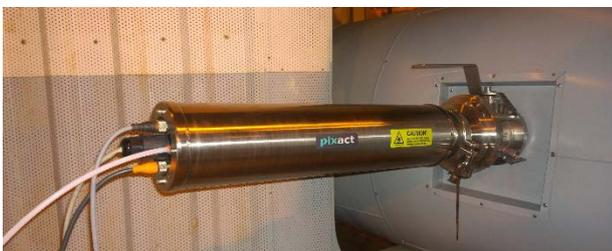
Figure 6. Pixact Bubble Monitoring system installed on the reactor inlet
