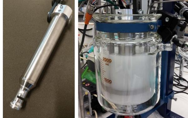
Figure 4. PCM probe for laboratory-scale reactors
