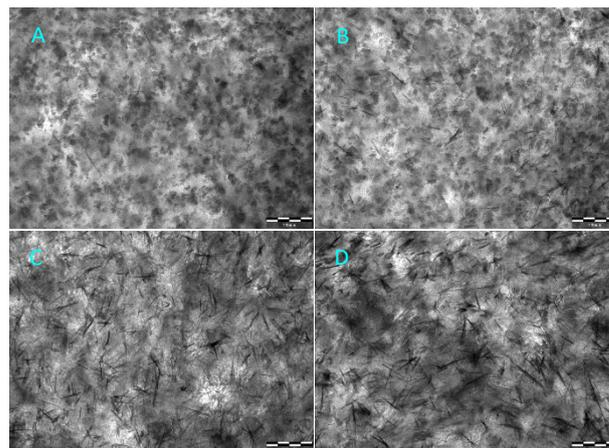
Figure 1. Images taken during DCPD precipitation. A=first stick-like DCPD crystals among HAP; B=Growth phase, C=HAP has disappeared, D=final crystals. The pictures are taken at the points indicated in Fig. 2. 200 µm scale bar.
