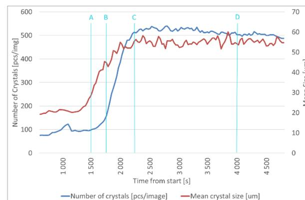
Figure 2. DCPD precipitation trends for the size and number of crystals
